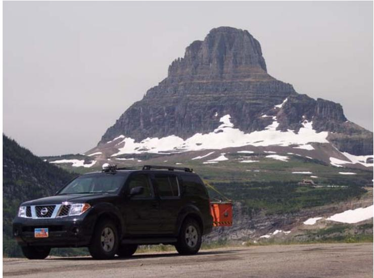
**1.0 GHz air-coupled antenna on high-speed pavement survey
