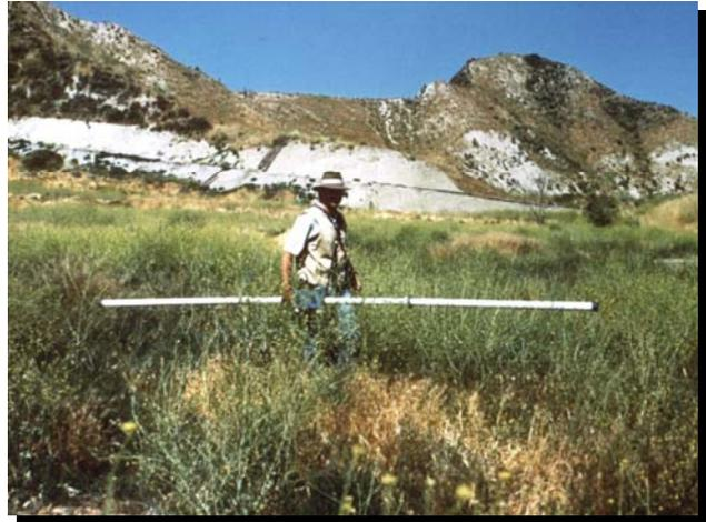
**Geonics EM-31 Terrain Conductivity Meter**
