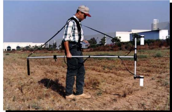
**Geometrics G858 Cesium Magnetic Gradiometer**
