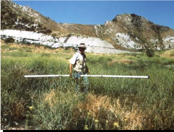
Geonics EM-31 Terrain Conductivity Meter
