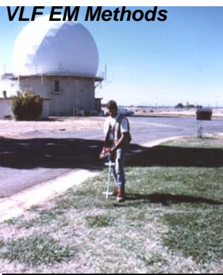
Metrotech Utility Locator
