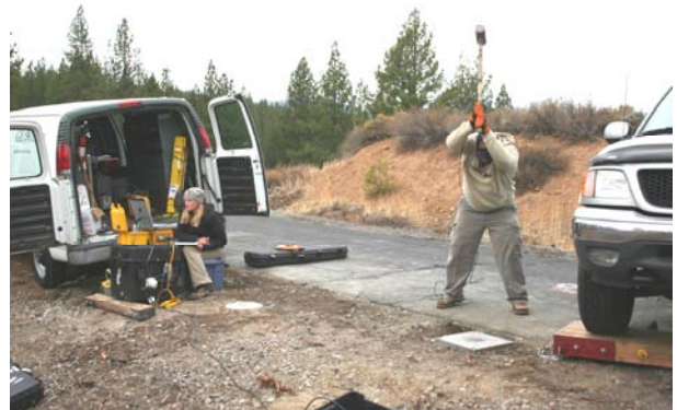
Standard source is a person with a sledge hammer, shown here making a P-wave (note heavy shear plank – 140Kg plus vehicle)
